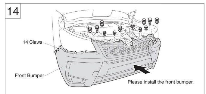
Before reinstalling the front bumper, reconnect the fog lamp connectors.
