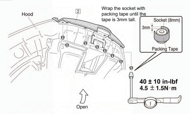
Do not allow any of the nuts to drop into the engine compartment.
